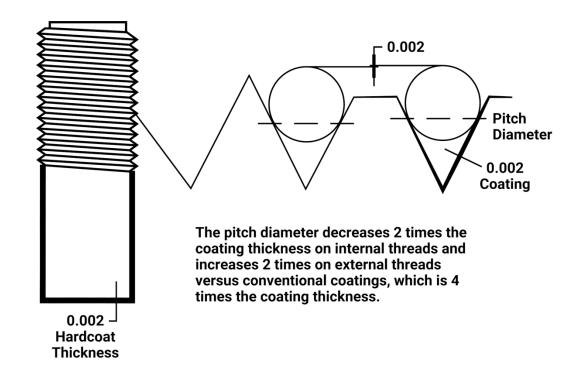
When a "V" thread is to be cut, allow for hardcoating by using the formula: build-up  $\times$  4. This will equal the pitch diameter change. A typical example is: Desired P.D. = .405/.4091 (7/16 N.F. Internal Thread) Coating thickness .002 +/- .0002 (.001 +/- .0001 build-up). Minimum build-up is .0009 x 4 = .0036 P.D. change; Maximum build-up is .0011 x 4 = .0044 P.D. change. Machine P.D. to .4094/.4127
